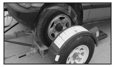
**Step 9.** While tightening straps, pull cross strap forward to ensure even tightening. Tighten straps until each tire starts to flatten against tire stop. After each strap is tight, insert a safety pin in each winch. Disengage towed vehicle parking brake.
